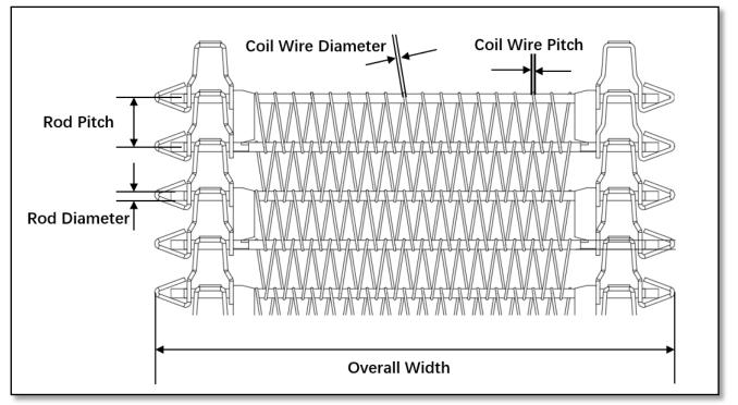
**NOTE:** When measuring Coil Wire Pitch, it is best practice to measure over 10 pitches and then divide by 10 to obtain the average pitch.
